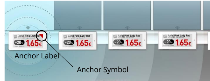
[Signal strength measurement between an Anchor label and a label]
